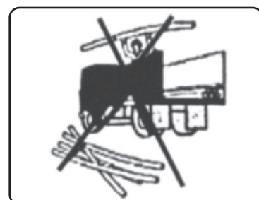
Figure 3: Unloading by using timber slides
